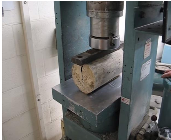
Fig 2: Split Tensile Strength Test of Cylinder
