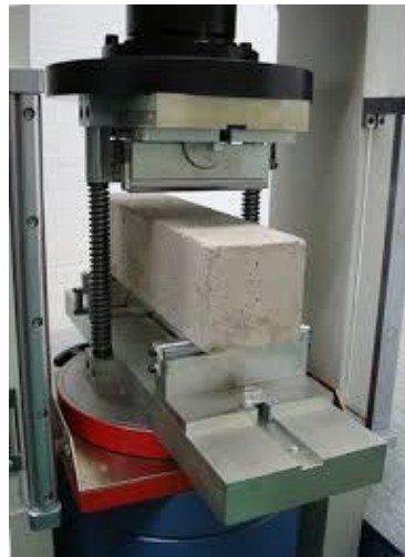
Fig 3: Flexural Strength Test of Beam
